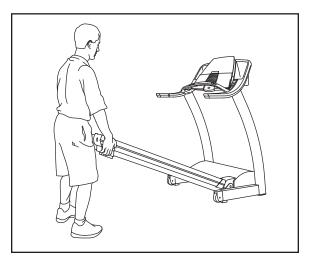
2. Hold the treadmill frame firmly with your left hand. Using your right hand, pull the latch knob to the right and hold it. Raise the frame until the pin on the latch knob is aligned with the hole in the left handgrip. Then, release the latch knob. Make sure that the latch knob is fully released so the pin is fully inserted into the hole in the left handgrip.
